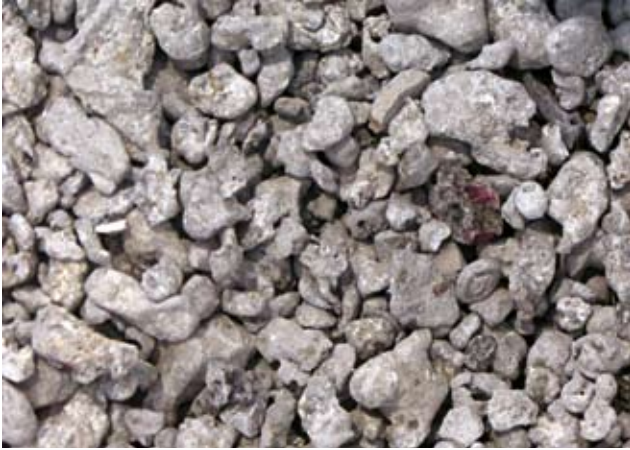
7 Aluminiumfraktion 8,0–35,0 mm • Aluminium fraction 8.0–35.0 mm
