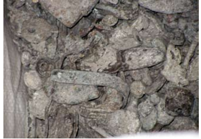
8 Kupferfraktion 8,0–35,0 mm • Copper fraction 8.0–35.0 mm
