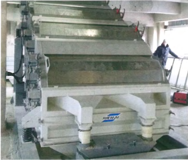
Figure 4. RHEWUM WAF installed at Agropolychim plant.
